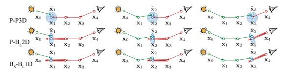
Figure 2.1: An example how the volumetric photon density estimators (shown P-P2D, P-B<sub>1</sub>2D, B<sub>s</sub>-B<sub>1</sub>1D) can be applied on different vertices along a path (the path is located entirely in a medium).
