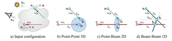
Figure 1.1: Illustration of the used volumetric radiance estimators.
