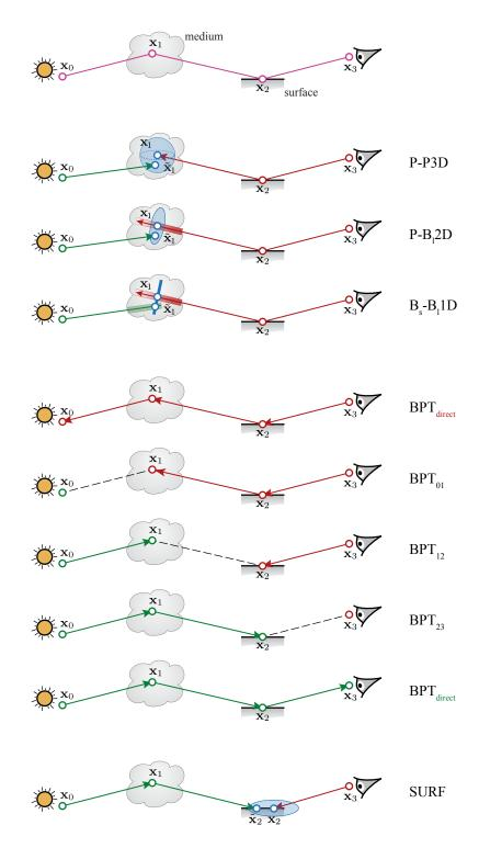
Figure 2.2: An example of *all* estimators along a fixed path. The path has 4 vertices (i.e. its length is 3), one of the two inner vertices is located in a medium, the other on a surface. Therefore, there are 7 volumetric density estimators, 5 path integral estimators and one surface photon density estimator. Only 3 volumetric photon density estimators are actually shown as the others differ only in a beam type and their image would be very similar.
